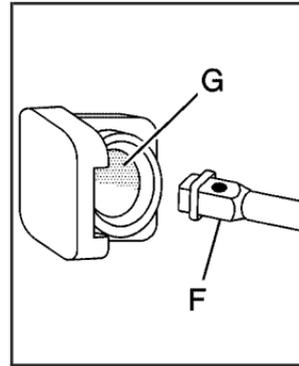
4. Insert the hoist end (F) through the hole (G) in the rear bumper and onto the hoist shaft (E).
