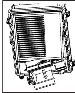
1. Locate the air cleaner/filter assembly. See *Engine Compartment Overview* on page 506.
