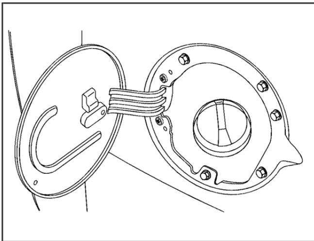
The tethered fuel cap is located behind a hinged fuel door on the driver's side of the vehicle. If the vehicle has E85 fuel capability, a yellow cap with the words "E85 / Gasoline" can be seen.
