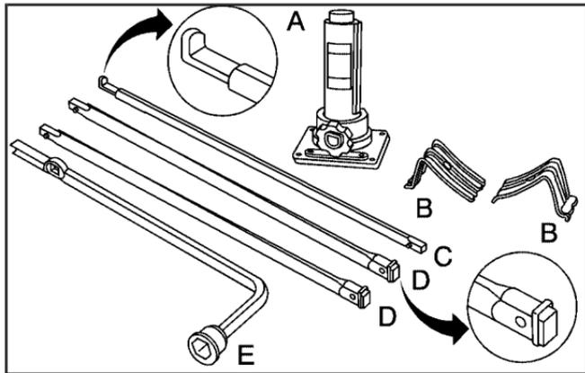
The tools you will be using include the jack (A), the wheel blocks (B), the jack handle (C), the jack handle extensions (D), and the wheel wrench (E).
