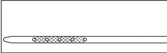
If the oil is below the cross-hatched area at the tip of the dipstick, you need to add at least one quart/liter of oil. But you must use the right kind. This section explains what kind of oil to use. For engine oil crankcase capacity, see *Capacities and Specifications on page 626*.
