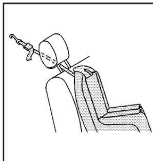
If the position you are using has an adjustable head restraint and you are using a single tether, raise the head restraint and route the tether under the head restraint and in between the head restraint posts.
