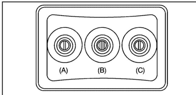
The A/V jacks, located on the rear of the floor console, allow audio or video signals to be connected from an auxiliary device such as a camcorder or a video game unit to the RSE system. Adapter connectors or cables could be required to connect the auxiliary device to the A/V jacks. Refer to the manufacturer's instructions for proper usage.
