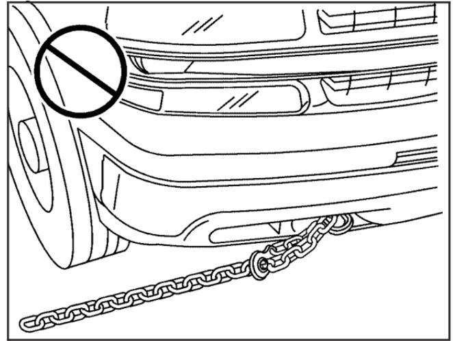
**Notice:** Never use recovery hooks to tow the vehicle. Your vehicle could be damaged and it would not be covered by warranty.
