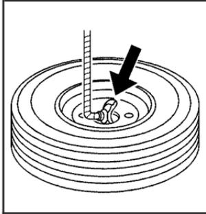
2. Tilt the retainer downward and through the wheel opening. Make sure the retainer is fully seated across the underside of the wheel.
