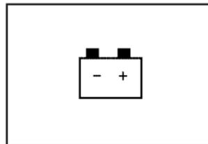
If this light comes on when the engine is running, there could be a problem with the charging system.
