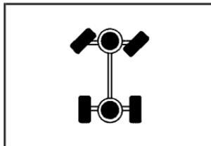
The four-wheel-drive light comes on when you shift a manual transfer case into four-wheel drive and the front axle engages.
