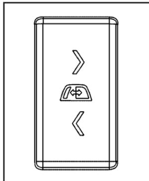
On vehicles equipped with a power sliding rear window, the switch is located in the overhead console.
