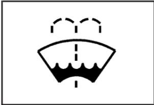
Open the cap with the washer symbol on it. Add washer fluid until the tank is full. See *Engine Compartment Overview* on page 506 for reservoir location.
