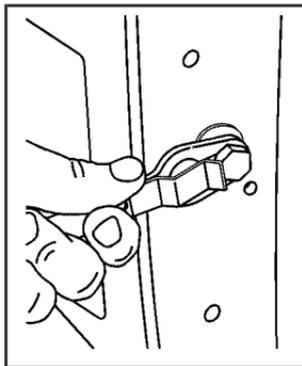
1. Raise the tailgate slightly and release both retaining cable clips. To release the retaining cable clips, lift the cable so it points straight out. Lift the clip over the bolt, and push the cable forward then rotate down.
