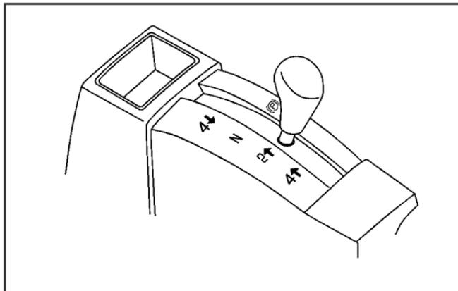
The transfer case shift lever is on the floor to the right of the driver. Use this lever to shift into and out of Four-Wheel Drive.
