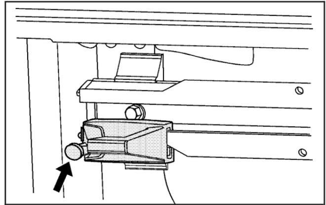
To adjust a tie-down, pull the locator pin out and move the tie-down to another location making sure the locator pin lines up with a locator hole on the rail. If the locator pin does not line up with the locator hole, the tie-down may be installed incorrectly. Turn it over and reinstall. Once the pin is inside the hole, the tie-down will not move side to side. The maximum load for each rail is 500 lbs (227 kg).
