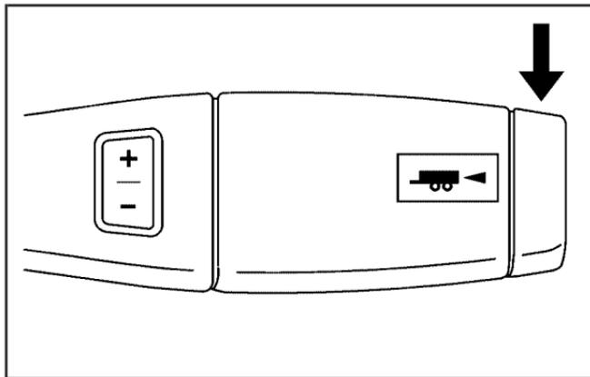
If your vehicle has an Allison or Hydra-Matic® 6-speed automatic transmission®, it has a tow/haul mode. The tow/haul mode adjusts the transmission shift pattern to reduce shift cycling, providing increased performance, vehicle control, and transmission cooling when towing or hauling heavy loads.
