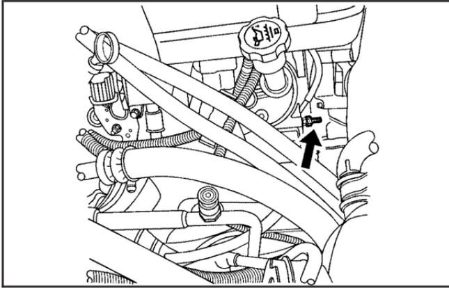
The remote negative (-) terminal is a stud located on the right front passenger side of the engine, where the negative battery cable attaches.
