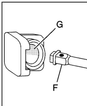
3. Insert the hoist end (open end) (F) of the extension through the hole (G) in the rear bumper.
