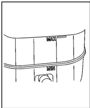
The fluid level should be above MIN. If it is not, have the brake system checked to see if there is a leak.
