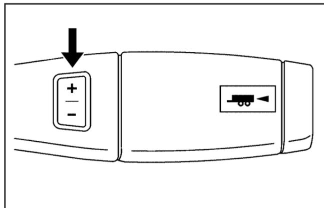
Your vehicle may have a Range Selection Mode. The Range Selection Mode helps control the vehicle's transmission and vehicle speed while driving down hill or towing a trailer by letting you select a desired range of gears.
