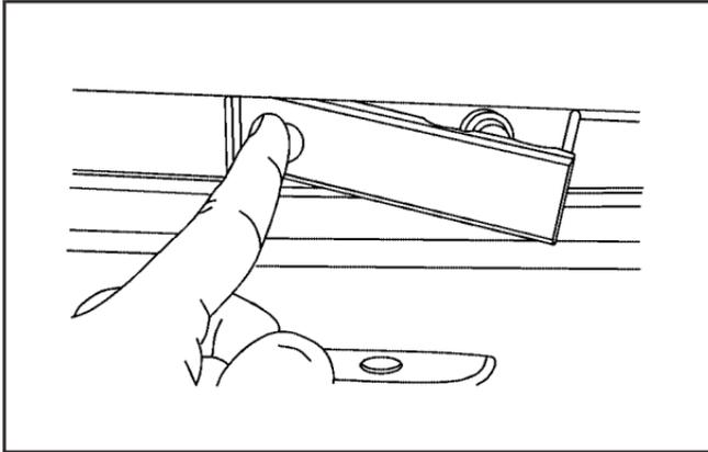
To open, press and hold the driver's side of the handle in and pull out on the exposed portion of the handle.
