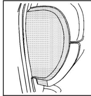
The instrument panel fuse block access door is located on the driver's side edge of the instrument panel.
