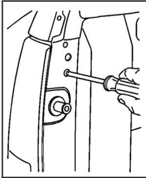
2. Remove the two rear lamp assembly screws near the tailgate latch strikerpost and pull out the lamp assembly.
