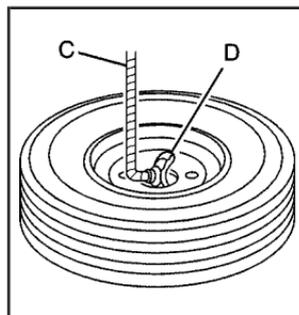
6. Tilt the retainer (D) at the end of the cable (C) when the tire has been lowered, so it can be pulled up through the wheel opening.
