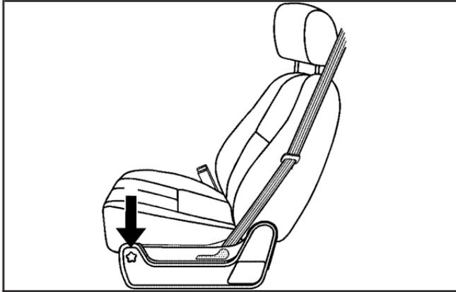
If your vehicle has this feature, the knob is located on the front of the driver seat lower cushion on the outboard side. Turn the knob forward to increase, and rearward to decrease lumbar support.
