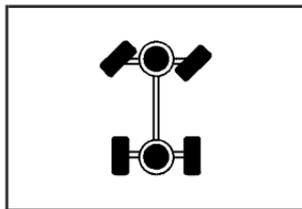
A Four-Wheel Drive indicator light comes on when you shift into four-wheel drive and the front axle engages. See *Four-Wheel-Drive Light* on page 271
