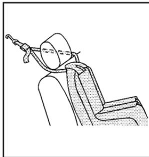
If the position you are using has an adjustable head restraint and you are using a dual tether, route the tether around the head restraint.
