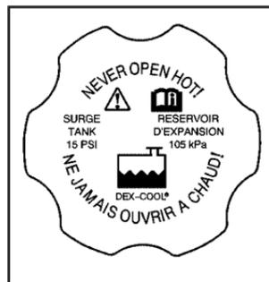
1. Remove the coolant surge tank pressure cap when the cooling system, including the coolant surge tank pressure cap and upper radiator hose, is no longer hot.
