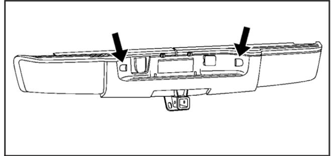
2. Turn the bulb socket counterclockwise and pull the bulb socket out of the connector.
